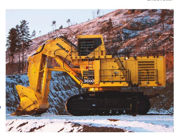
Even in confined work sites, you can maintain high production. The PC3000 is a powerful, versatile machine with advanced technology and a 16m3 shovel and 15m3 backhoe capacity, and the reach to fill 85-165 st trucks.
