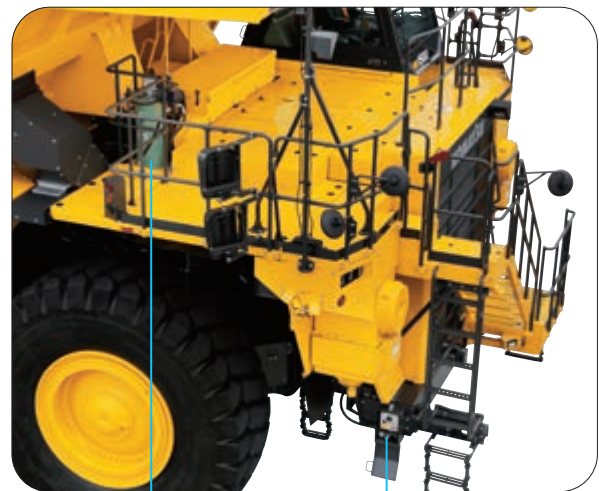
Grease pump pump and reservoir
