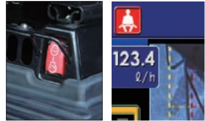
Secondary engine shut down switch and seat belt caution
