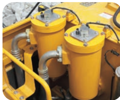
Clogging detector in hydraulic return filter prevents damage of hydraulic system
