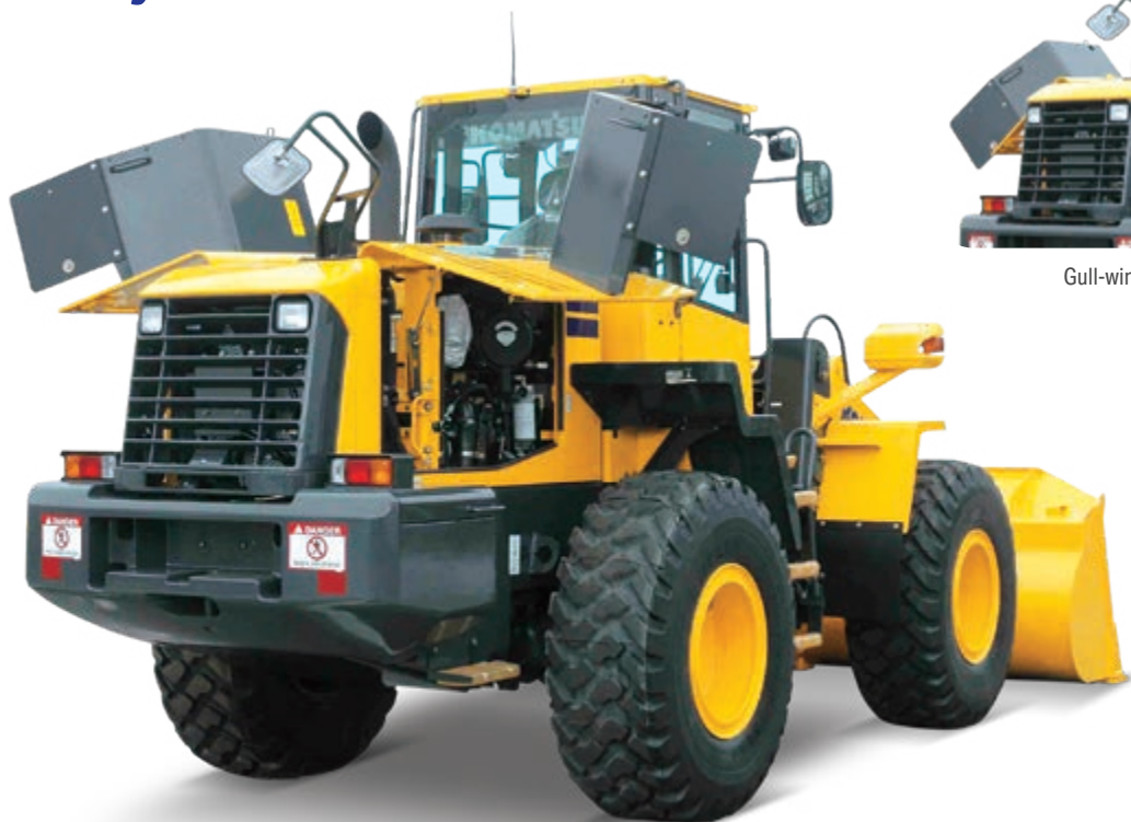
Gull-wing side doors upper locked position
