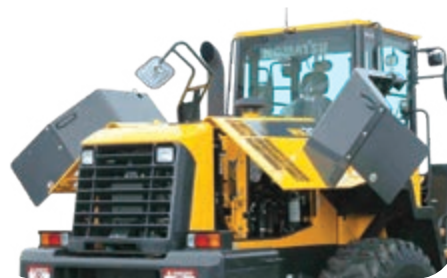
Gull-wing side doors lower locked position
