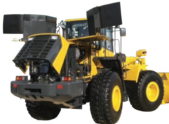
Gull-wing doors upper stop position
