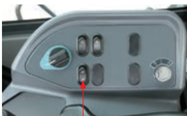
Dual mode engine power selection switch
