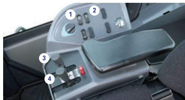
1: Cut-off ON/OFF switch 2: Cut off adjustment switch 3: Boom control 4: Bucket control
