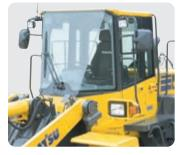
largest in its class providing maximum space for the operator. Increased seat slide adjustment to to the rear by introducing front mounted air conditioner unit.
