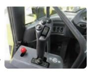
in loading operations. This system allows you to change the direction of travel and gear shifting with push buttons on the joystick. And you may pre-select the steering speed in 2 stages, depending upon whether fast V-loading or precise load & carry is required.
