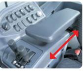
and distance to the sliding console and the large armrest can be adjusted for maximum comfort. Furthermore, the system is isolated from any vibration and shock from the loader equipment.
