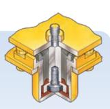
The large cab is mounted with Komatsu's unique ROPS/FOPS viscous mounts. The low-noise engine, hydraulically driven fan, and hydraulic pumps are mounted with rubber cushions. The cab sealing is improved to provide a quiet, low-vibration, dustproof pressurised, and comfortable operating environment. Also, the exterior noise level is the lowest in its class.
