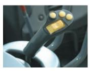
machine steering angle is exactly the same as the lever tilt angle.
